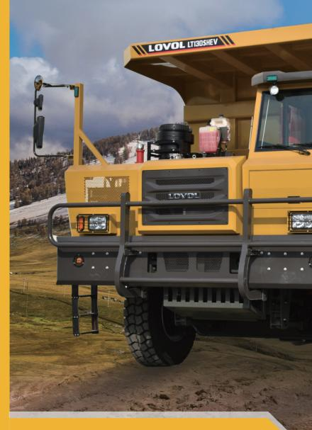
Curb weight (kg):50600 Max. gradeability (%):30 Engine Power (kW):426
